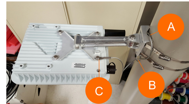
Figure 15: Attaching the security cable
